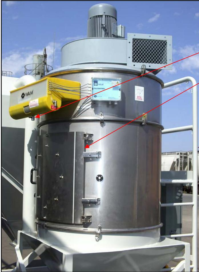
The WAM 400 Pulse jet dust collector runs all the time during operation. The pulse jet timing is preset and will need no adjusting in the field.
