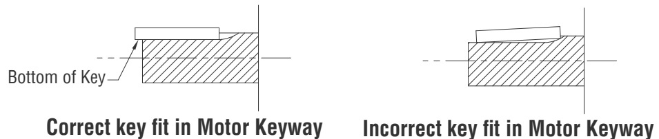
Figure 5 - Clamp Collar Motor Key Fit
