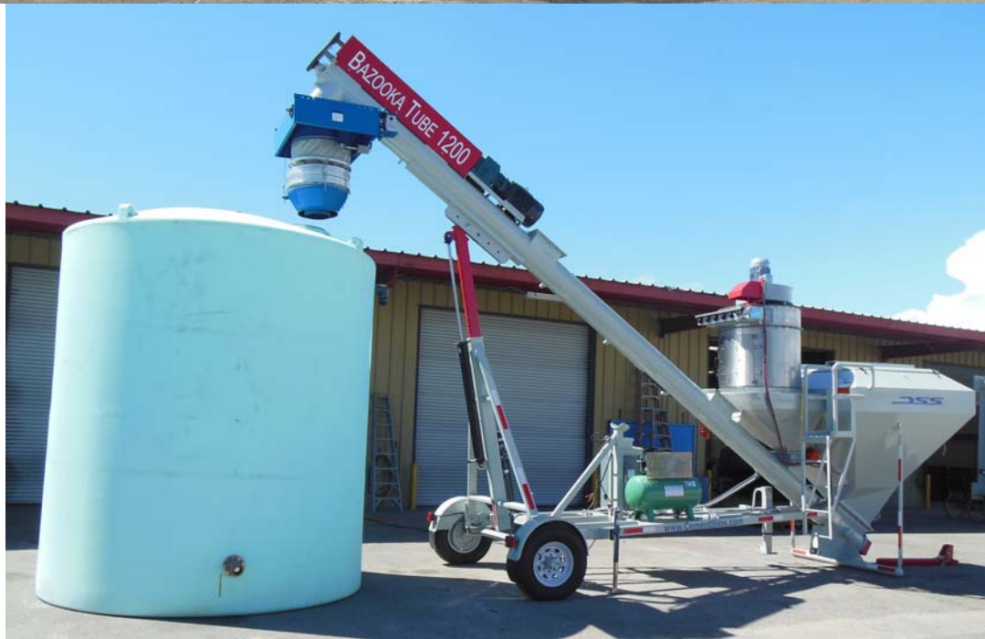
Loading Configuration to Truck or Mix Tank.
